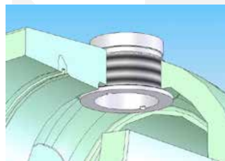
Flat surface formed in the vessel shell - reduces counter boring
