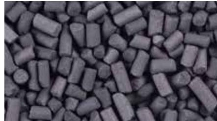
Ketones and terpenes are usually removed by activated carbon filters. Measuring VOCs with the BioSENSE before and after the biogas pre-treatment system provides you several options for minimizing expenses for activated carbon:
